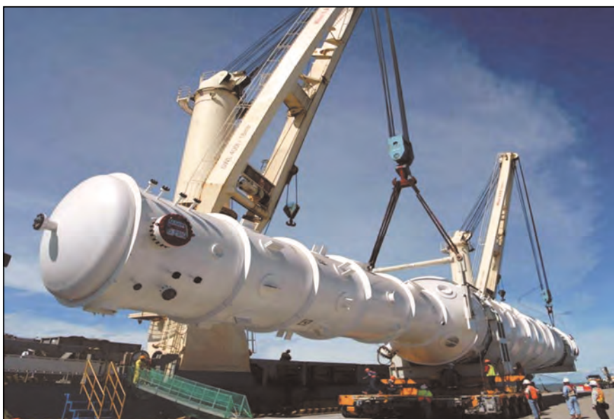
Plate 4.8 A cryogenic heat exchanger being unloaded
