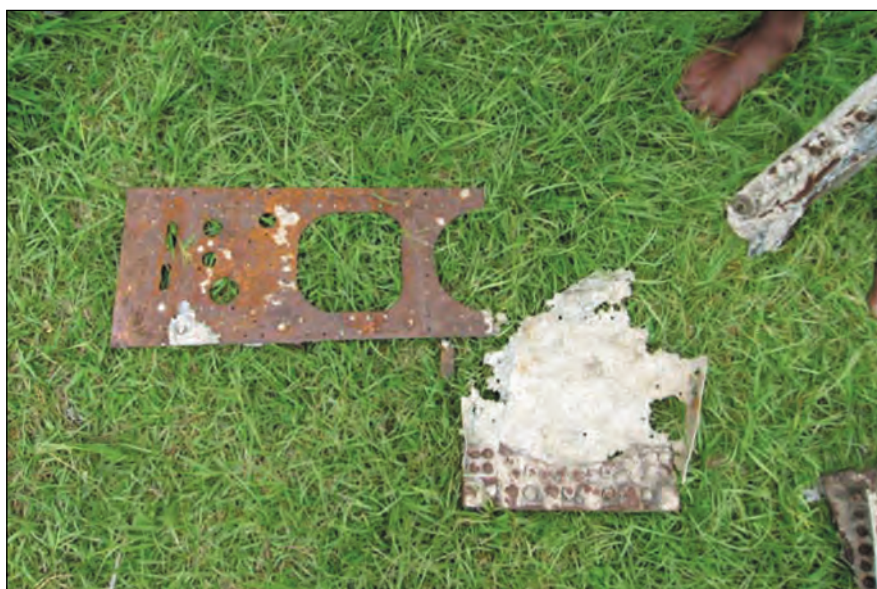
Plate 16.15 Instrument panel and aluminium skin from Japanese Zero fighter at Lea Lea
