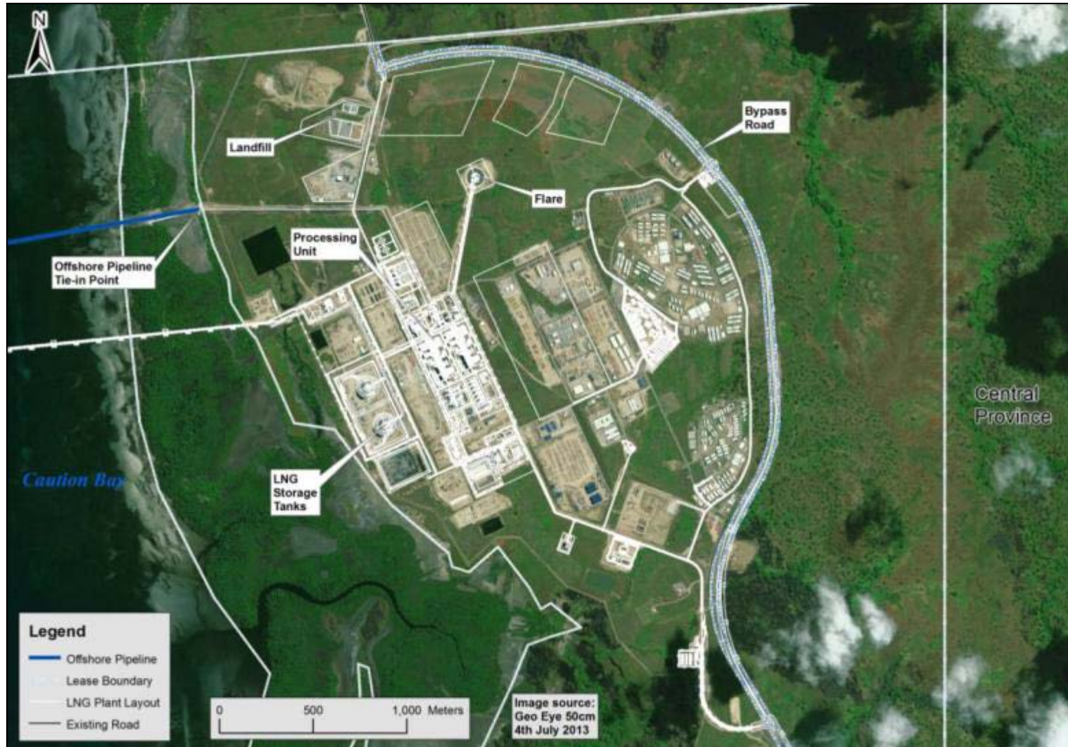
Figure 5-1: LNG Plant layout
