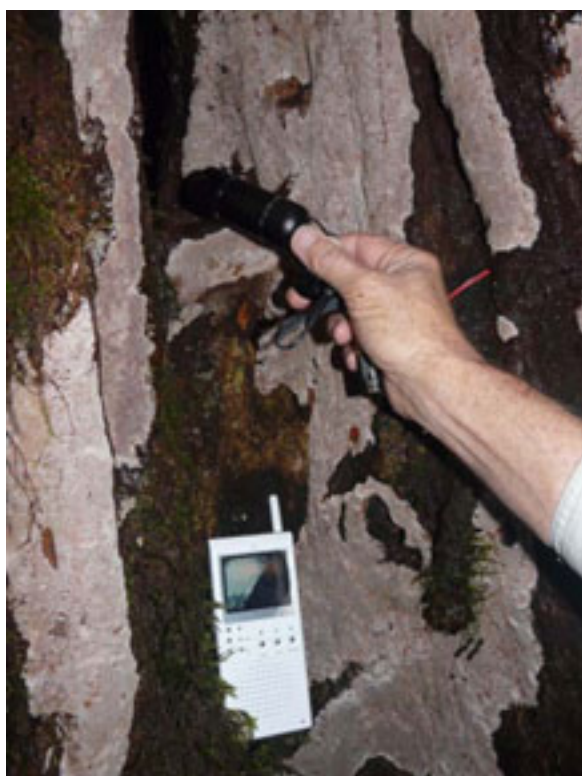
Figure 10 Transmitting video camera and portable television monitor used to inspect potential roost hollows for bats.
