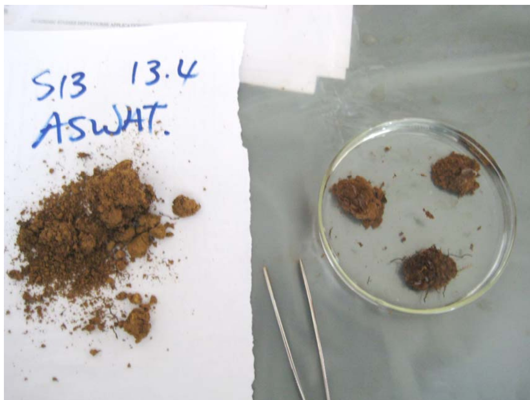
Plate 4 Aggregate stability in water test (ASWAT)
