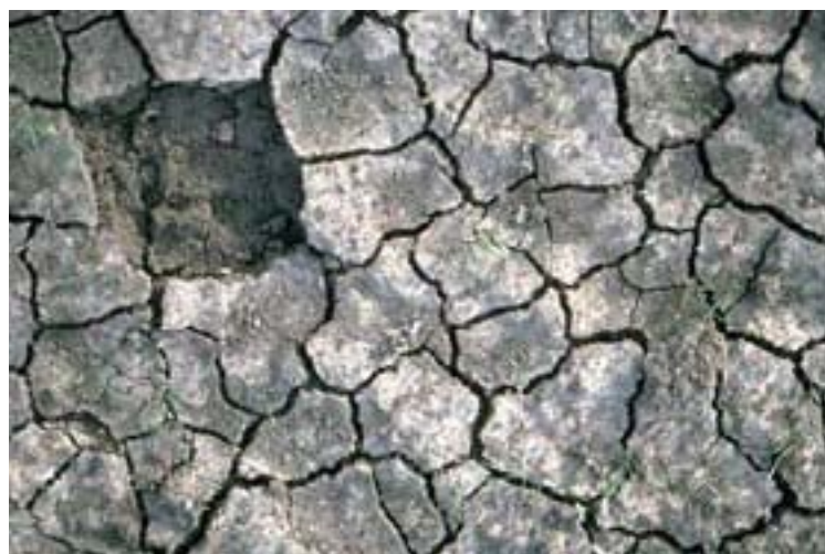
Plate 5 Surface crusting on a dispersive clay soil
