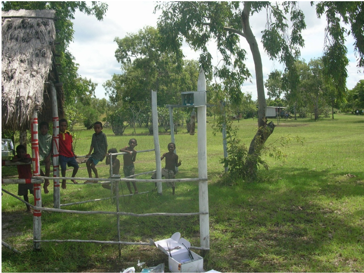
Plate 1. Showing Radiello passive monitor at Site A mounted near top of white post in centre of picture
