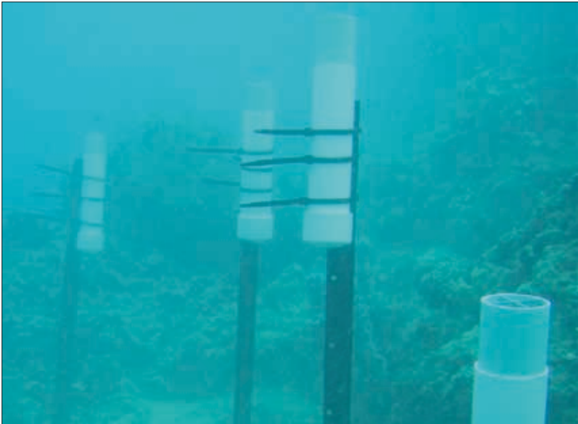
Plate 3.04 Group of installed sediment traps
