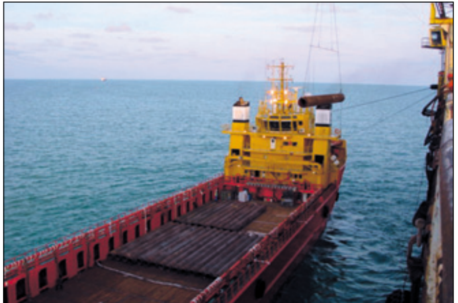
Plate 3.16 Typical pipe supply vessel, showing pipe sections on deck and a pipe section being transferred to the pipelaying vessel by crane
