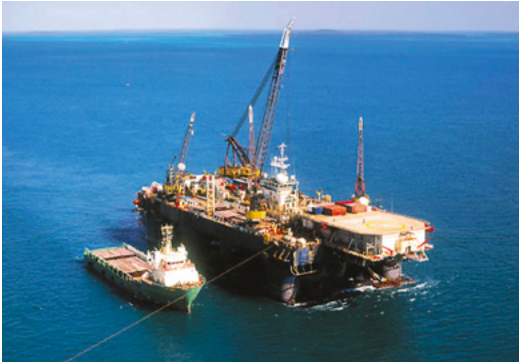
Typical anchored laybarge (above) and pipe supply vessel.
