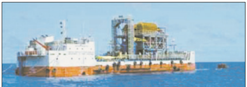
Plate 4.6 Barge-mounted desalination plant
