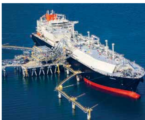
Loading of the first cargo on the second custom-built PNG LNG vessel, the Kumul
