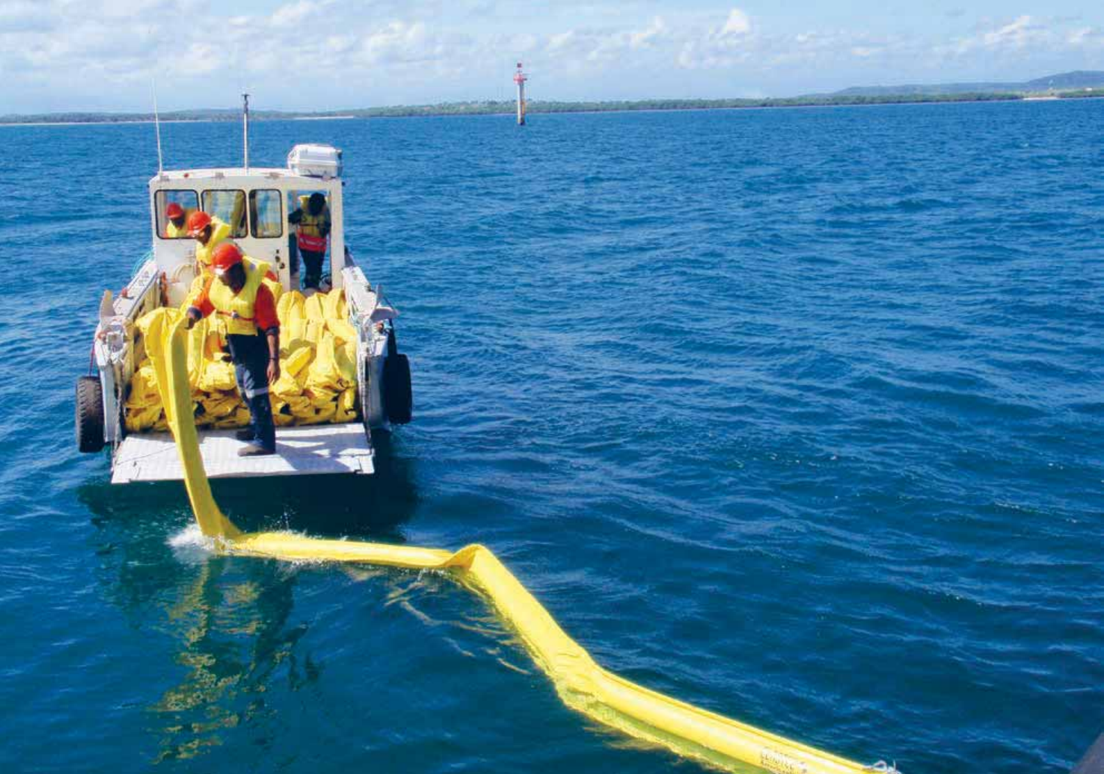
Plate 6.7 – EMPNG’s Emergency Response team practicing shallow water boom deployment
