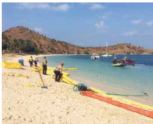
Plate 6.6 – Deploying a shoreline protection boom and skimmers during an emergency response exercise
