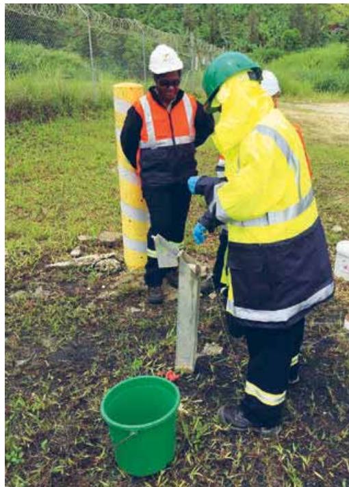
Plate 6.5 – Purging a groundwater sampling bore at the HWMF to allow for more representative sampling of groundwater conditions
