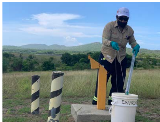
EMPNG Field Environmental Specialist, Isabel Roandi-Eka, conducting groundwater sampling at the LNG Plant site
