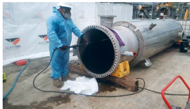
HGCP Mechanical Technician, Desmond Nombon, cleaning the monoethylene glycol regeneration package distillation column at the HGCP
