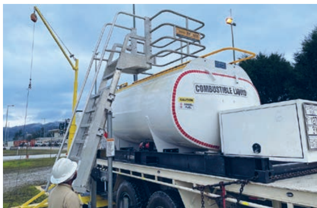
EMPNG’s Human Performance approach led to an innovative use of specialty ladders to reduce fall exposure for workers
