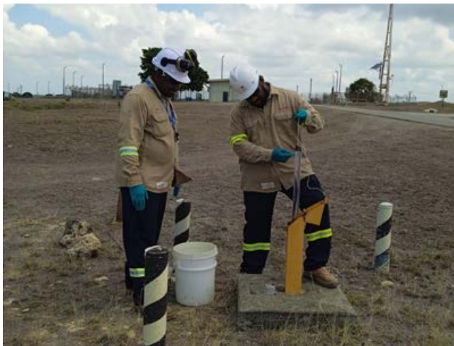
Field Environmental Advisors, Vincent So-on and Murithi Sari, conduct groundwater monitoring at the LNG Plant
