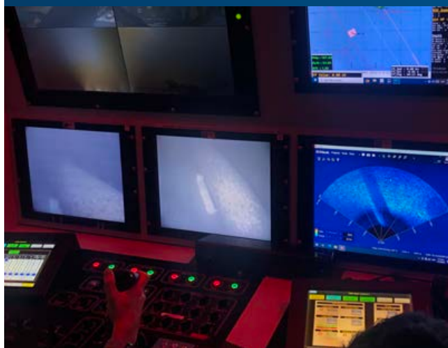
Footage from a remotely operated vehicle used to install grout bags to support the offshore pipeline
