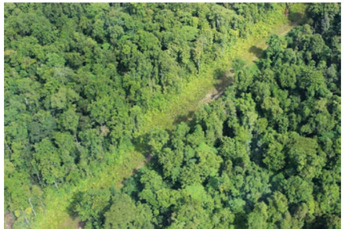
A reinstated section of the main onshore pipeline ROW
