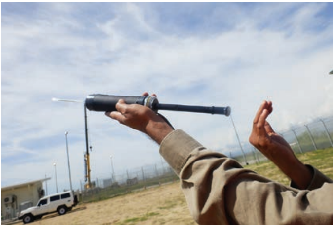
Demonstrating the use of a Gastec Sampling Pump in air quality monitoring
