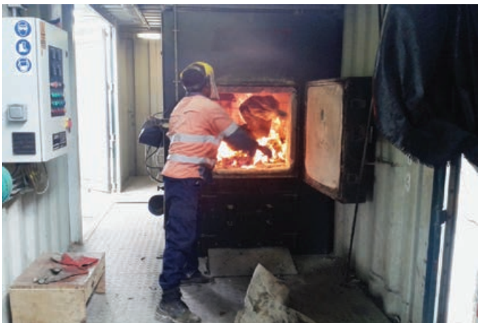
Moro Camp 5 incinerator operator disposing of dried sludge bags
