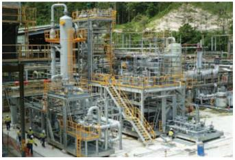
Plate 2.6 - Triethylene glycol module
