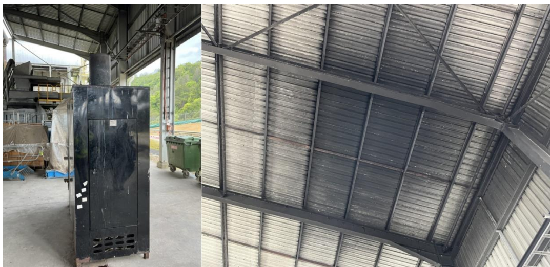
Figure 4.3: Improperly Ventilated Mediburn Incinerator at HWMF
