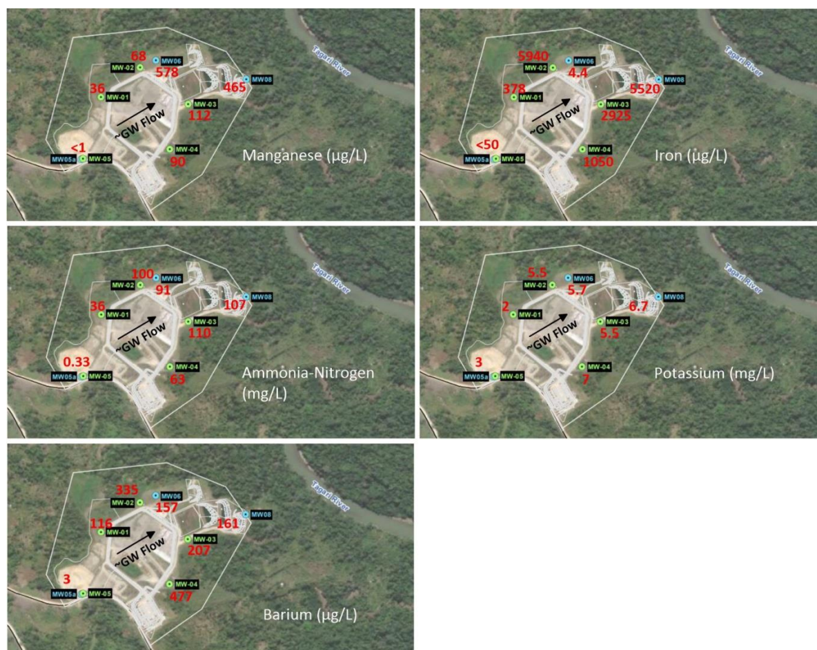
Figure 4.4: Average 2023 Concentrations of Main Leachate Parameters in Groundwater at HWMF
